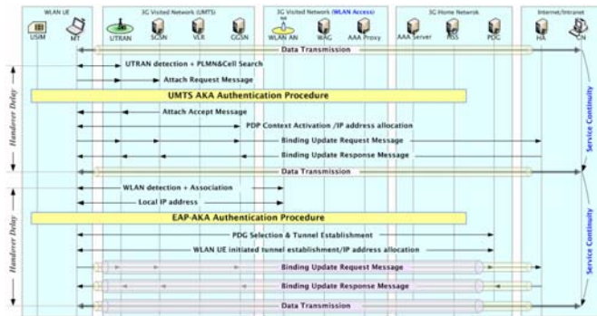
Fig. 4. UMTS to WLAN handover procedure
