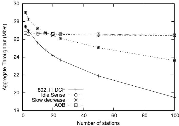
Fig. 1. Aggregate throughput vs. number of stations,  $BER = 10^{-5}$
