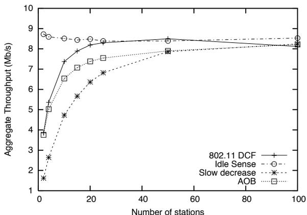
Fig. 4. Aggregate throughput vs. number of stations,  $BER = 10^{-4}$
